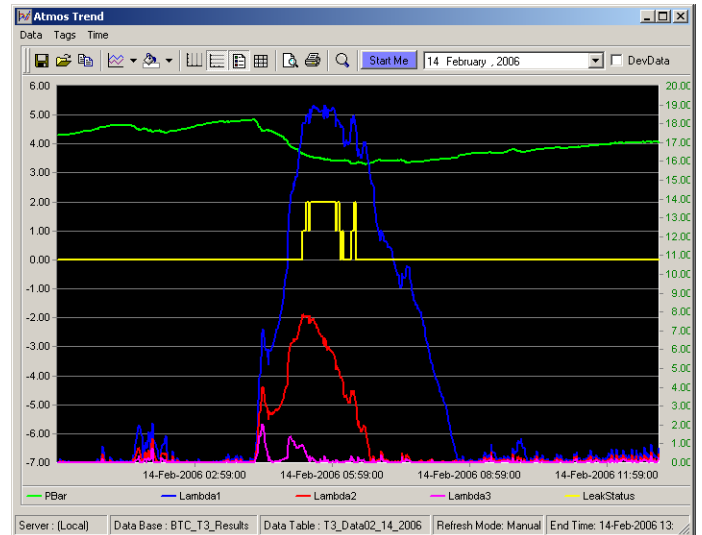
Figure 10: Trend displaying “line fill” LDS response Primary axis: Lambda variables and Leak Status (Yellow) Secondary axis: Average Line Pressure (Green)
