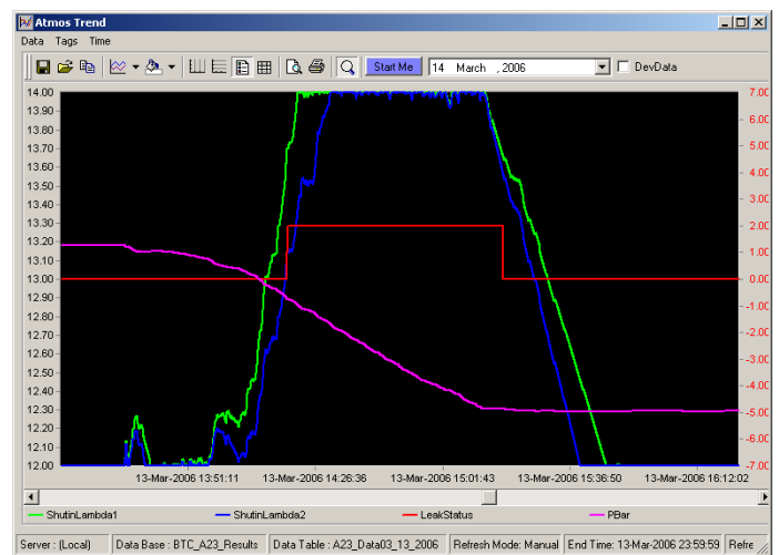
Figure 12: Trend displaying full section LDS response to a “simulated leak” under shut-in conditions Primary Axis: Average Line Pressure (Purple) Secondary Axis: Lambda variables (Blue and Green) and Leak Status (Red)
