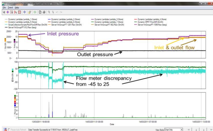
Figure 4 An example of the flow meter discrepancy change from -45 to 25 m 3 /h
