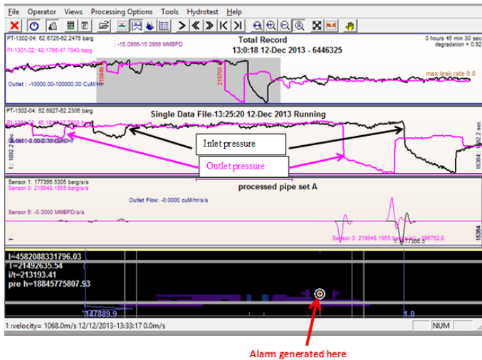
Figure 9 Leak test results showing the clear pressure responses to two leaks in the 234.5 KM segment
