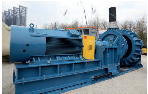
The MDR500 fits on a frame 1400 – the largest frame in the MD series to benefit from an innovative pump maintenance slide base
