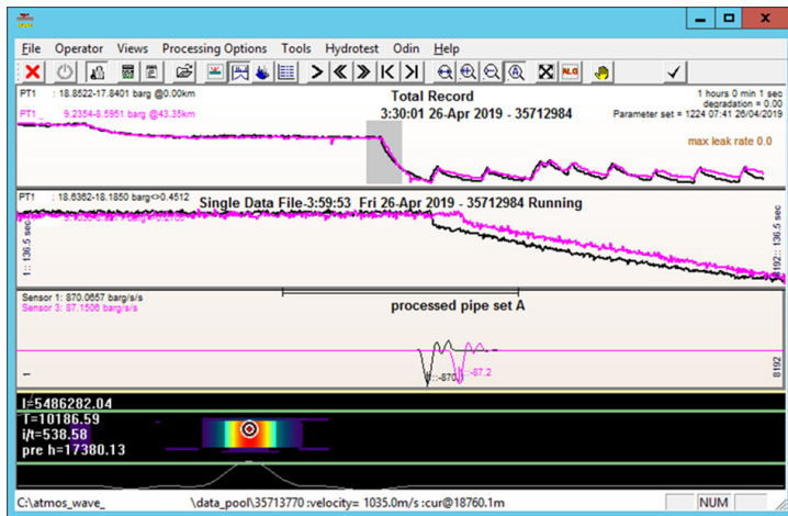
Figure 2. An example of a theft event generating 0.4 bar pressure drop.
