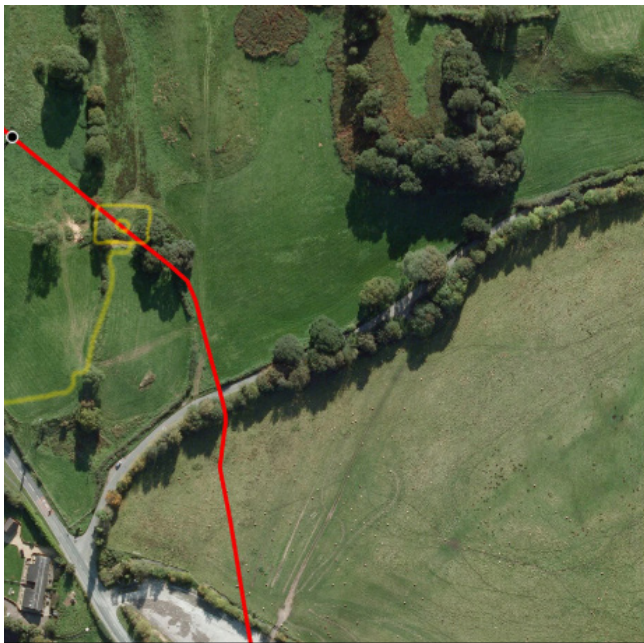
Figure 5. A double tapping point exposed by the pipeline operator following location provided by the leak detection system. The black dot is the location given by the theft detection system, the yellow dot is the actual tapping point, and the yellow line shows the hosepipe route.
