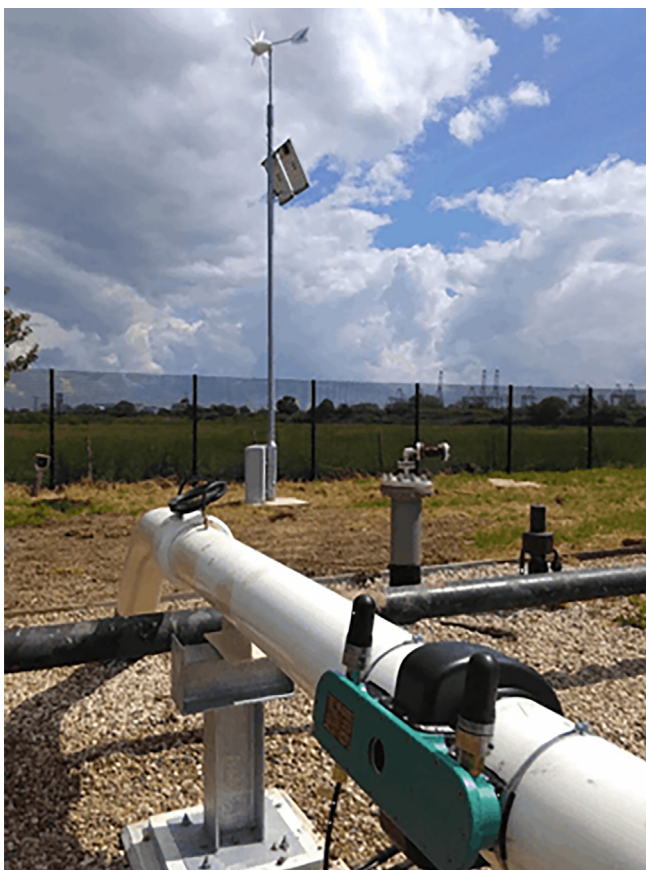
Figure 2. Atmos Eclipse in operation using solar and wind power in a remote location.
