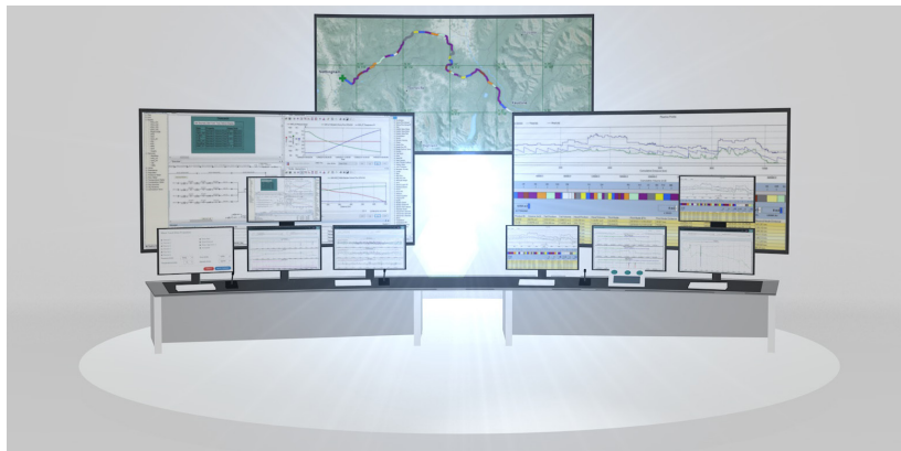
Figure 2. Atmos SIM can use data delivered from the field through a supervisory control and data acquisition (SCADA) system for advanced applications on a gas pipeline, such as leak detection and batch tracking.
