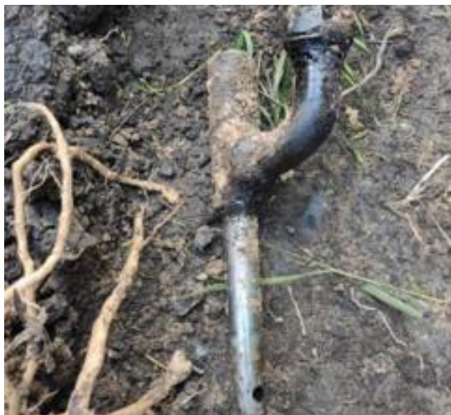
Figure 1. Metal spike embedded in a pipeline wall. These methods pose a high risk of leakage and environmental damage.
